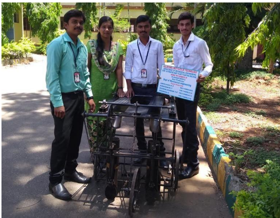
Semi automated baby plant planting machine
